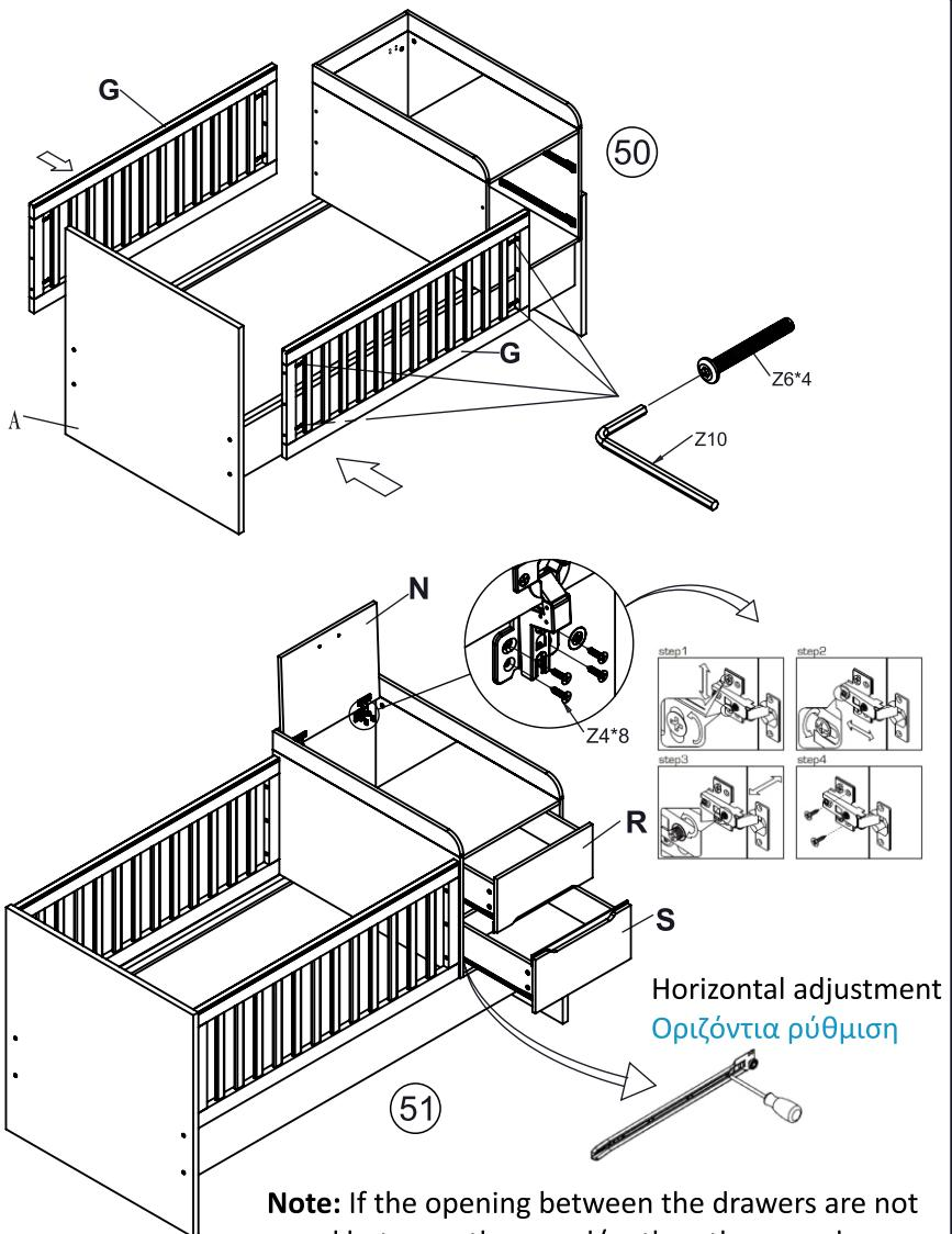
**Note:** If the opening between the drawers are not equal between them and/or the other panels, you can adjust this by changing the screw in the drawer conductor position as specified below.
